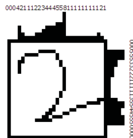
Figure 1. Histogram for digit 2. For each row and column we have counted the ink pixels.
